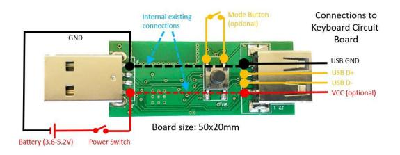
The size of the circuit board is 66x20mm with the two connectors, or 50x20 without. The thickness is 10mm with the connectors, or 3.5mm without the connectors and the mode button.
